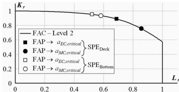
Fig. 12 FAPs of critical crack lengths
