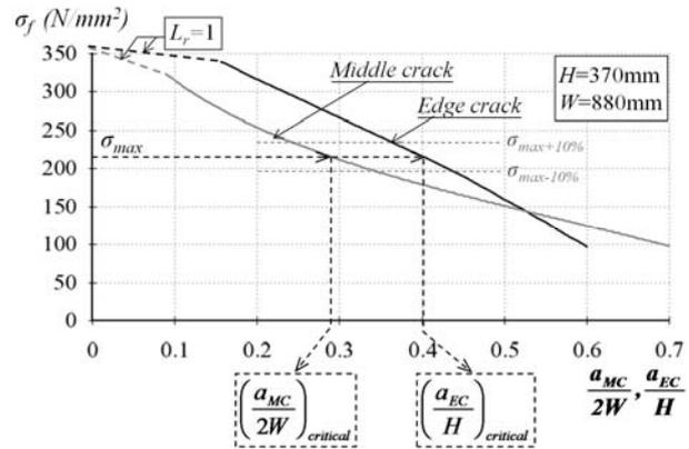
Fig. 10 Failure stress of SPE located in the deck
