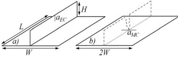
Fig. 2 Stiffened plate element including a) an edge crack in the stiffener, b) a middle crack in the plate
