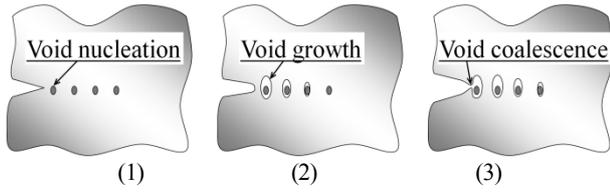
Fig.1 Three-stages ductile fracture behaviour
