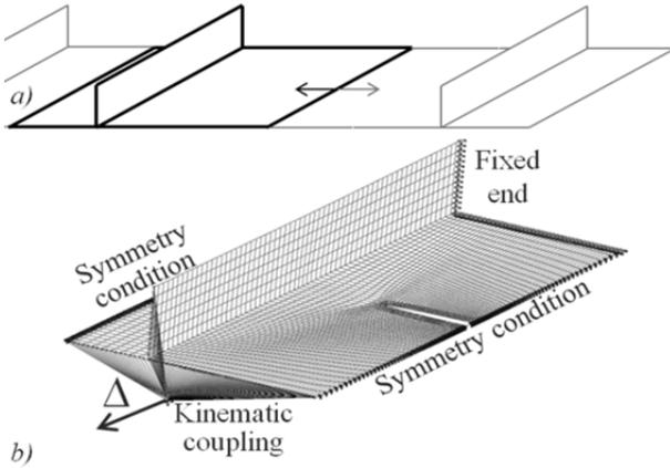
Fig. 7 SPEiMC finite element modeling
