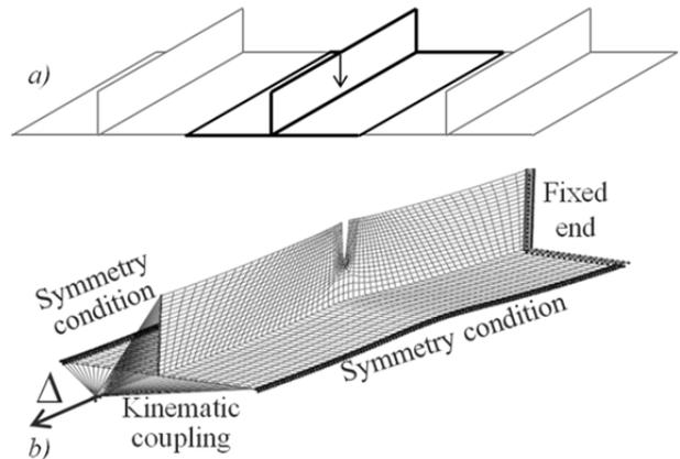
Fig. 6 SPEiEC finite element modeling
