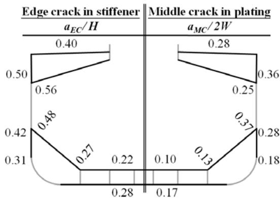
Fig. 13 Nondimensional critical crack lengths in the midship section
