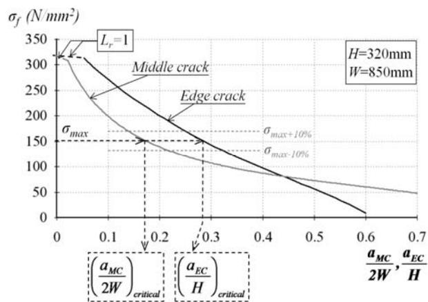
Fig. 11 Failure stress of SPE located in the bottom
