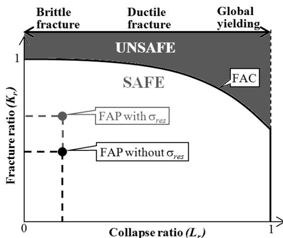
Fig. 3 Failure assessment diagram
